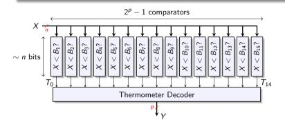
Thermometer decoder: counts the ones in a thermometer code.
