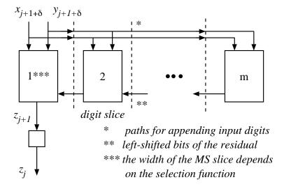
• Array (2D) organization: [2] If pipelined, Max throughput  $1/t_{slice}$
